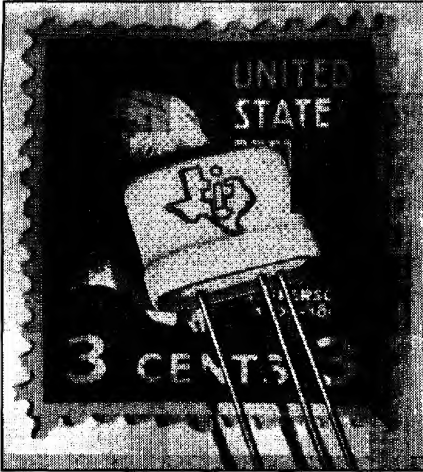
Left: The first commercial Si transistor from Texas Instruments (1954). Right: The first transistor pocket radio (1954). It had four Ge npn transistors.
